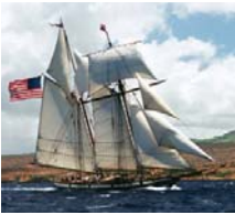
LYNX , Newport Beach, California Square Topsail Schooner, 122' sparred length, 23' beam, 94 gross tons Owner - Lynx Educational Foundation
