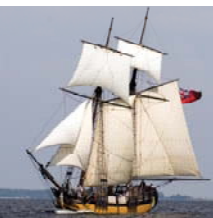
SULTANA , Chestertown, Maryland Square Topsail Schooner, two masts, 97' sparred length, 17' beam, 43 gross tons Owner - Sultana Projects, Inc., www.schoonersultana.com
